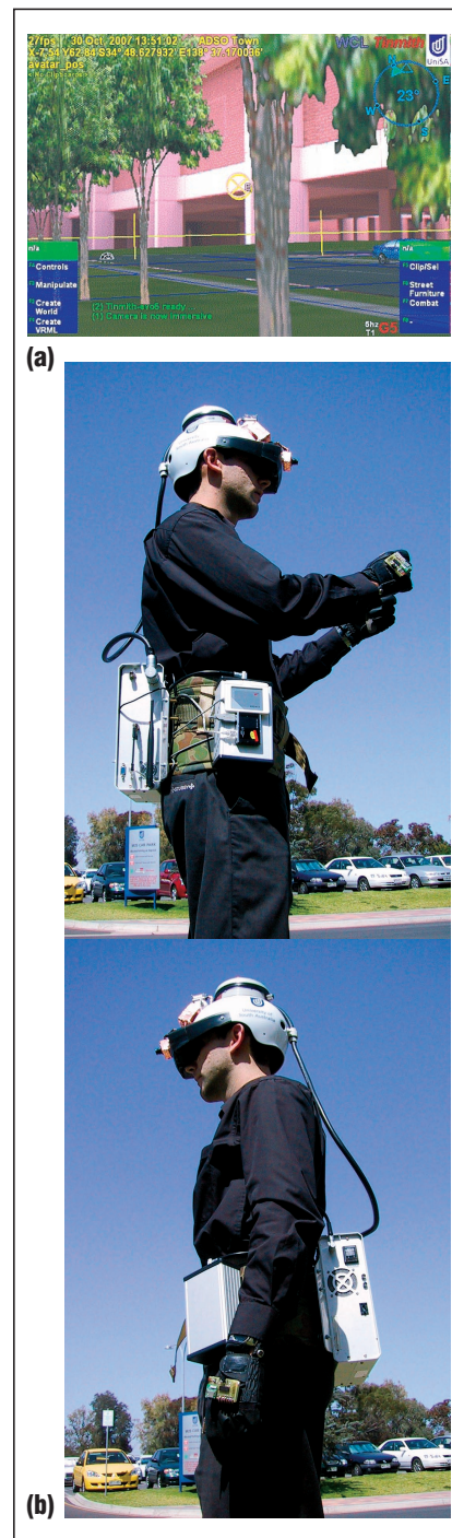
Figure 1. An example of wearable augmented reality: (a) a user's view through a head-mounted display and (b) a back and front view of our Tinmith system. Using the Tinmith system allows for full 3D rendering of computer-generated content. (photos courtesy of the Wearable Computer Lab, University of South Australia)
