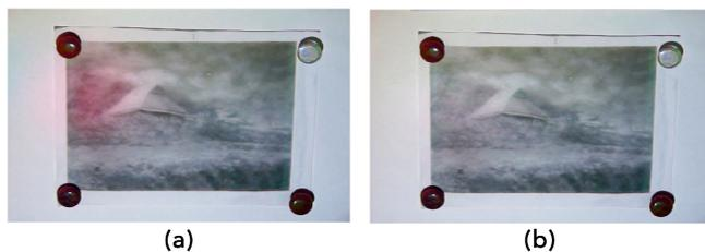
Fig. 18. Appearance control with the canceling of additional light. Our system can make the colored area appear monochromatic. (a) Instant at which a red spotlight illuminates the object surface and (b) after the system compensates to eliminate the red light.
