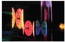
This saccade-based display is a device capable of presenting two-dimensional images using a unique bar of addressable light sources (a column of LEDs). In a dimly lit environment, each time the saccadic eye movement of the observer is detected, the flashing pattern of the column light expands, and ghostly images appear in midair.
