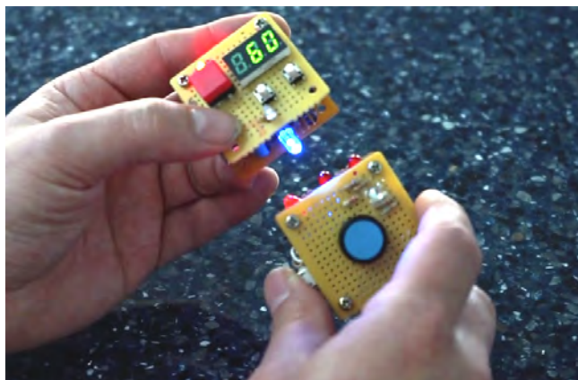
Figure 2. Modules connect in a network through outlets (blue LED) and inlets (red LEDs). Connections are made by holding an outlet near an inlet; the module cycles through the inlets to let users select a specific inlet. Through short range infrared communication, modules negotiate RF connection details. The LED is then lit solid, confirming an established connection. Disconnecting modules is achieved in a similar fashion, by again holding the modules together for a brief time.
