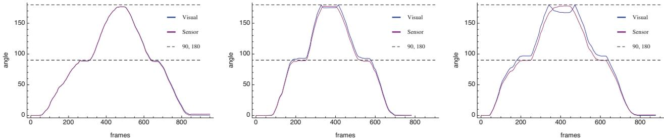
Figure 2: Angular measurements from the visual tracker and sensors for different distances from the axis of rotation. Left 0% offset, middle 5% and right 10%. Beyond 180°, the rotation is measured in the other direction and the angle decreases.
