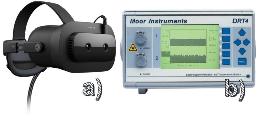
Figure 2: Experimental platform. a) Varjo XR-1, a Video See-Through Head-Mounted Display. b) Moor DRT4 to measure skin blood flow.
