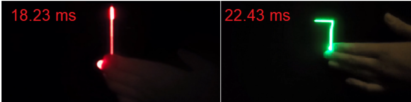
Figure 1: Our system enables interaction with laser graphics on moving objects with an end-to-end latency of 4 ms.
