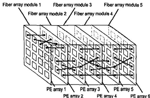
Figure 2 A Multi-stage interconnection network
