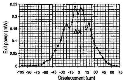
Figure 6 Alignment tolerance for a channel
