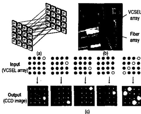
Figure 5 Interconnection topology and experimental results
