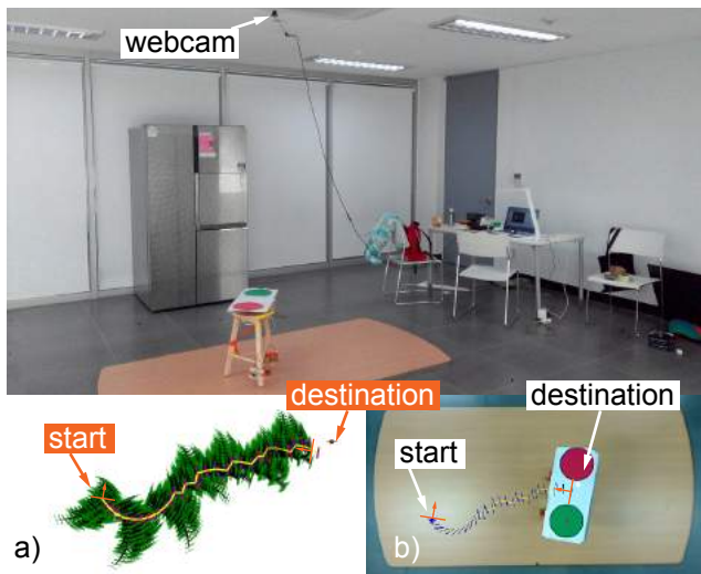
Figure 2: (a) offline breadth-first optimised path; (b) resulting real path after applying the sequence of vibration patterns
