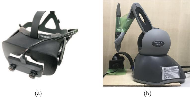
**Fig. 1.** Devices used in our AR-PETS: (a) the Oculus Rift with Ovrvision Pro attachment and (b) the Phantom Omni haptic device.
