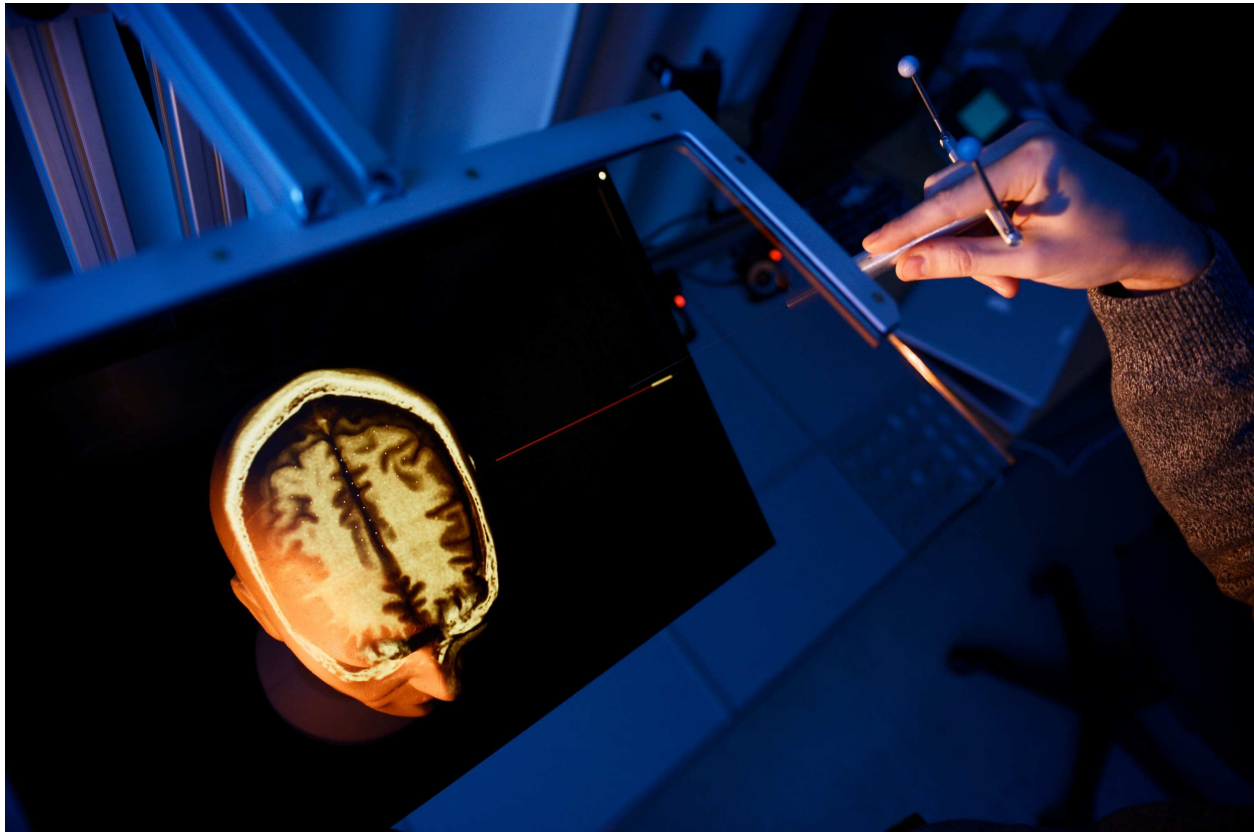
Fig. 3. A-me 's optical see-through AR display presenting a tomographic brain visualization mapped on a dummy head. © Mark Stegelman
