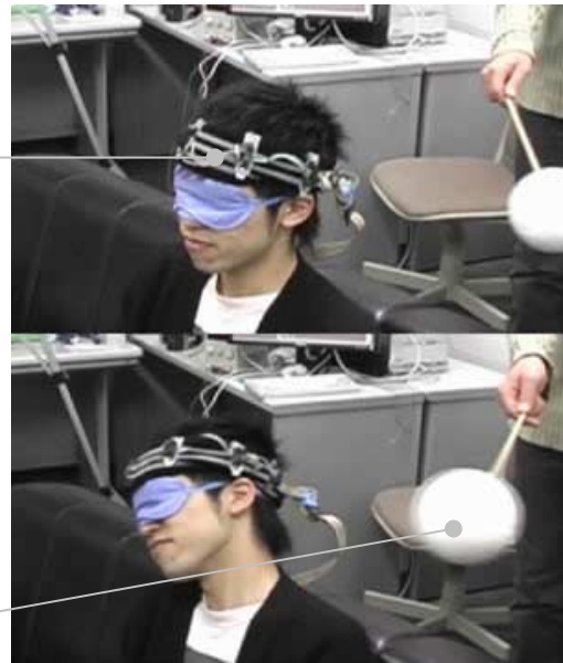
figure 2. The Haptic Radar device allowed wearers to move to avoid unseen stimulus approaching from behind.
