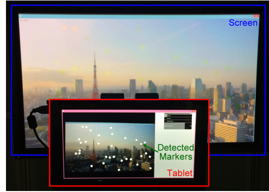
Fig. 3 Client application showing the dot pattern overlaid on the camera image.
