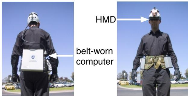
**Figure 3. TINMITH: Our previous high-fidelity prototyping platform for AR with a head-mounted display (HMD).**
