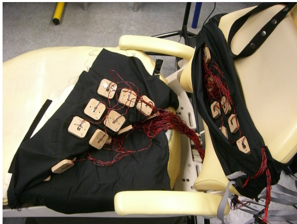
Figure 4. photograph of the vibrators inside the chair and the belt
